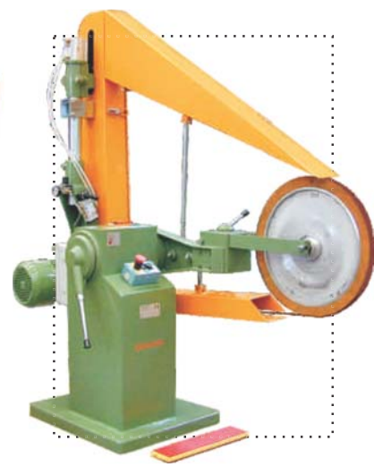
Special forks for the use of contact wheels up to 600 mm
