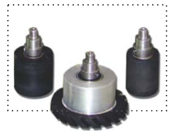
Contact rollers for overhang workings
